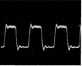
23 IC307 60 pin 3.6Vp-p, 49MHz
