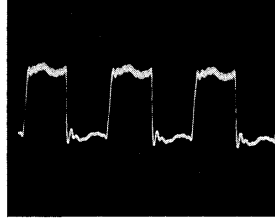
27 IC307 76 pin 5Vp-p, 1μs
