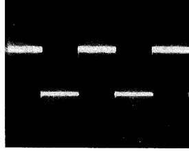
26 IC307 74 pin 6Vp-p, 0.1μs
